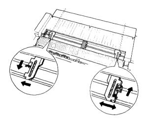
3. Slide the paper support to a point midway between the sprocket units.
